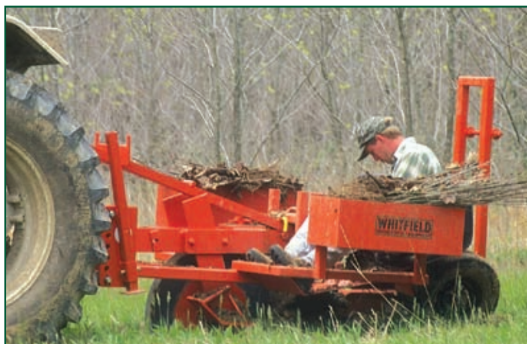
Figure 7. A mechanical tree planter suitable for planting large bare-root seedlings. (Photo courtesy of Ron Rathfon)
